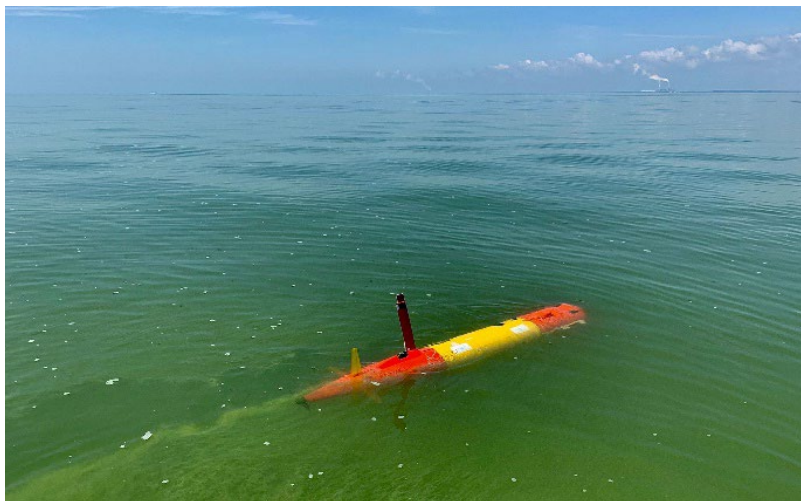
One of Monterey Bay Aquarium Research Institute's long-range autonomous underwater vehicles makes its way through the green, algae-rich waters of Lake Erie to track the 2019 harmful algal bloom as part of a research collaboration with NOAA. (Image: Ben Yair Raanan, Monterey Bay Aquarium Research Institute)
