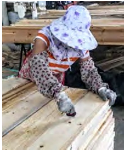
Chinese sawmill working shown applying a counterfeit grading mark to structural lumber. (photo: EBPA)
